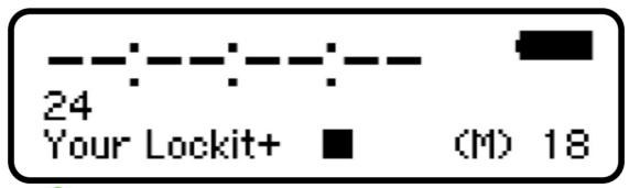
Press and hold UGreen to confirm the timecode and start the C-Jam.
