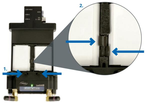
**Note:** To change batteries please push the battery release levers. Please assure to push the levers down before inserting the batteries.
