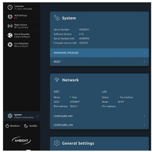
Drag and drop the latest firmware file (named "LP-X.X.X.upgrade") from your desktop. **Please note:** The Lockit+ needs to be externally powered to perform a firmware upgrade.
