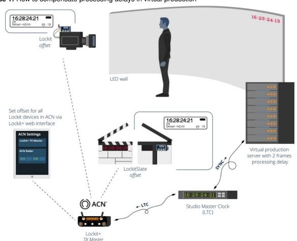
Use Case 2: Adjust internal processing delays of cameras – classic setup
