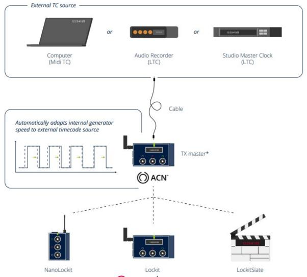
\* Can be any Lockit device started up with O Red + U Power. We broadcast Start, Stop and Freeze Frame through ACN.
