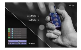
You can use your NanoLockit both as a Timecode Generator AND a Live Logger. The goal of the Logging feature is to mark good and bad clips (or several parts of a clip) directly on set. This can save loads of time in post-production.
