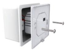
4. Align the top part of the front panel with the back panel and connect them back together, then replace the fixing screw at the bottom.
