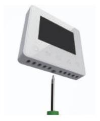
2. Connect the thermostat according to the wiring diagram.
