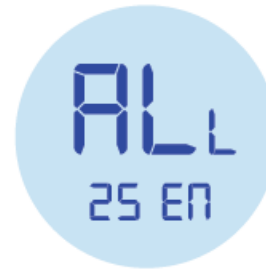
Air Sensor with Floor Limit (ALL)
