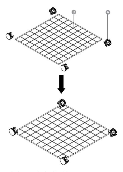
$\bullet$  Attach 4 connectors  $\underline{\mathbb{A}}$  to four corners of a wire grid panel  $\underline{\mathbb{B}}.$
