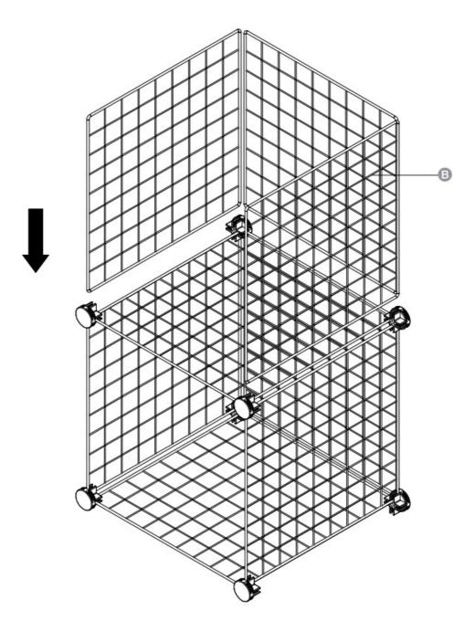
• Insert three grid panels B into connector slots.
