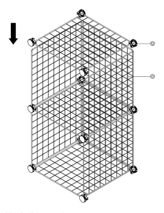
$\bullet$  Add grid panel  $\, \underline{\! B \!\!\! B }$  to cube with 4 connectors  $\, \underline{\! A \!\!\!\! A }$  .
