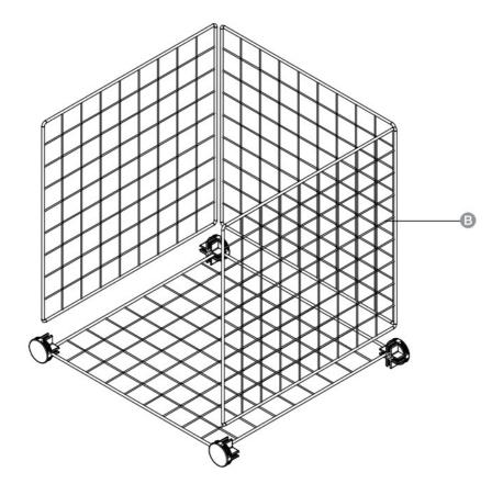
$\bullet$  Add three grid panels  $\ensuremath{\mathsf{B}}$  into connector slots.
