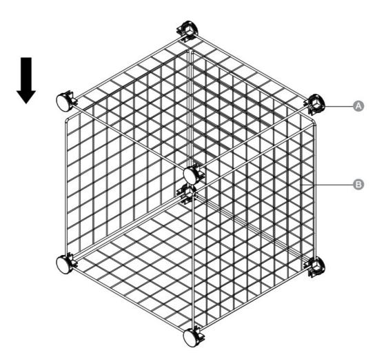
• Attach 4 connectors  $\[ A \]$  to grid panel  $\[ B \]$ . Attach grid panel to the top corners of the cube.
