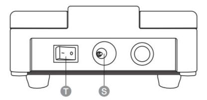
• Connect the adapter (AB) to a power outlet and the other end to the power socket (S). The LED lights up.
