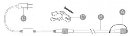
A Female cord connector C Attachment plug with fuse
