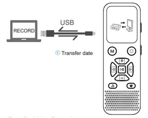
Use the supplied USB cable to connect the recorder with your computer, then you could see the recorder disk in your computer just like a normal usb disk.
