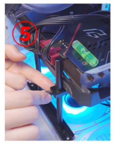
6. Tighten the screws (self-tapping screws Need to tighten forcefully).
