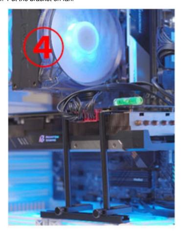
5. Slide the braces to the below of GPU, tighten screws after confirming level.
