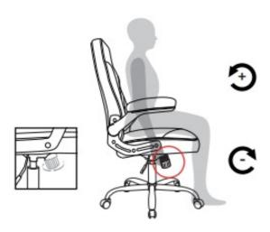
To increase tension: While seated, turn knob forward (Counter clockwise). To decrease tension: While seated, turn knob backward (Clockwise). Set the tilt tension to control the resistance you feel when leaning back.
