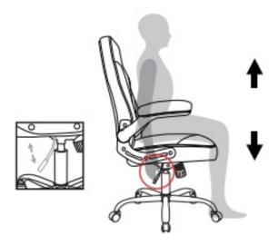
To raise:While taking your weight off chair, lift lever up. To lower:While seated, lift lever up
