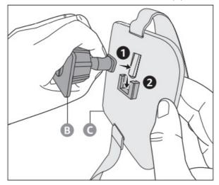
2. Attach the other end of swivel mount (B) onto the back of the mirror (A).
