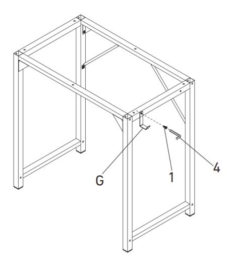
Attach Hook (G) to the Leg (D) with Screw (1)\*1.
