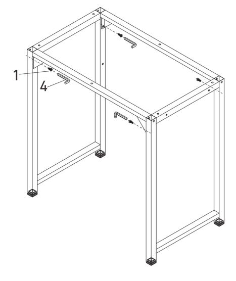
Secure the remaining four screw holes of the Crossbars (B&C) completely to the installed Desk Frame with Screws (1)\*4.
