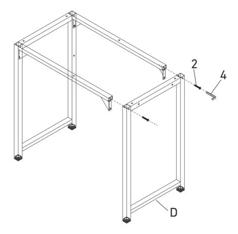
Attach Leg (D) to the installed Desk Frame with Screws (2)\*2. Please make sure the Legs are oriented correctly.
