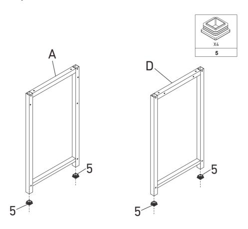
Attach Foot Pad (5)\*4 to the four feet of the Legs (A&D).
