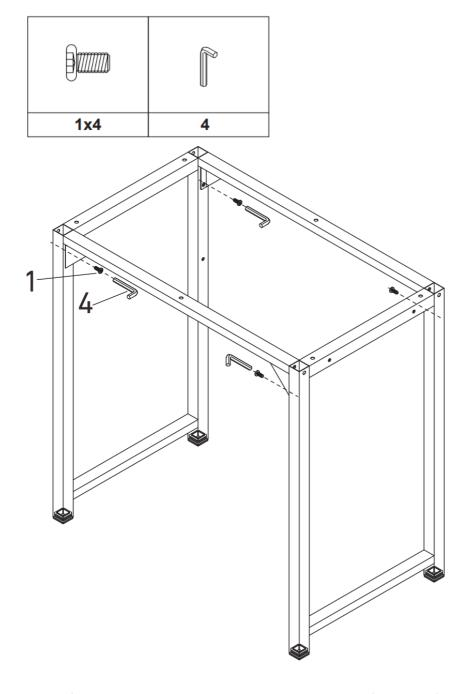
Attach Crossbar (B) to the front side of the Leg (A) and Crossbar (C) to its back side with Screws (2)\*2.
