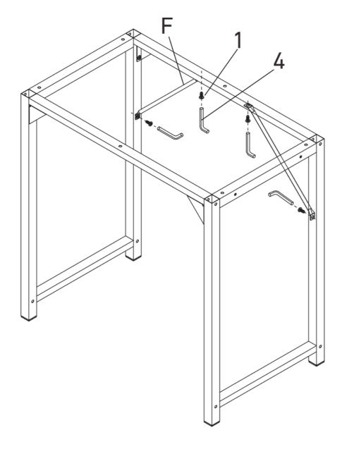
Attach Bar (F)\*2 to the Legs (A&D) and Crossbar (C) with Screws (1)\*4.
