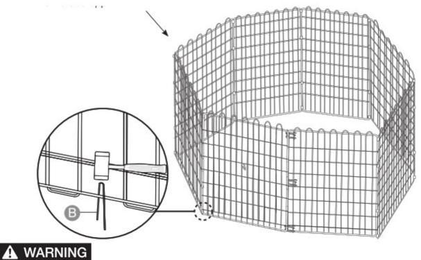
For outdoor installation, use a rubber mallet to secure the pet pen to the ground with the stakes (B) on the edges of each panel.
