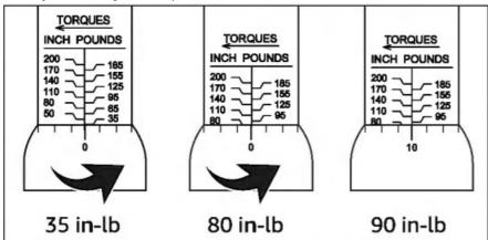
**Example:** Setting the torque to 5.65 Nm
