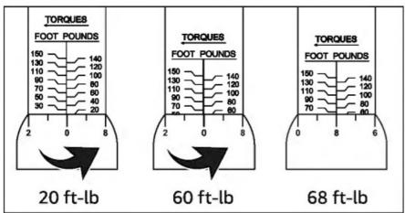
**Example:** Setting the torque to 94.9 Nm
