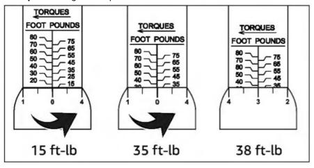
**Example:** Setting the torque to 47.5 Nm
