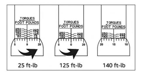
**Example:** Setting the torque to 101.7 Nm
