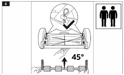
3. Align the roller shaft to the desired adjustment level, then refit the bolts, nuts and spacers .
