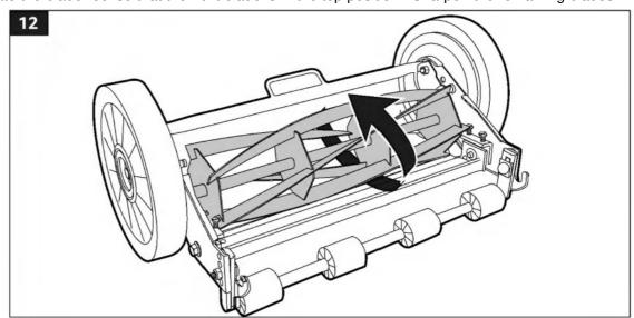
• To test for sharpness, turn the lawn mower upside down. Wearing gloves, take a strip of paper and carefully turn the blade reel so that a blade cuts a small portion of the paper. Repeat for all blades. Each blade should slice the paper evenly across the entire length of the cutter blade while the reel turns smoothly.
