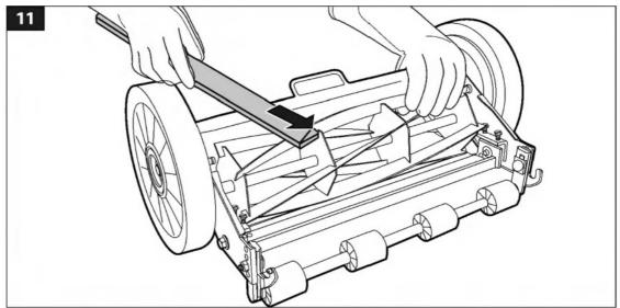
• Rotate the blade reel so that the next blade is in the top position . Sharpen the remaining blades.
