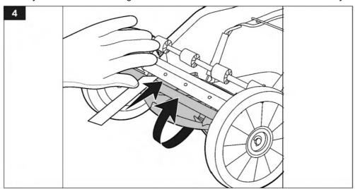
• t If the product has an intermittent cut, adjustment should be made to the appropriate side of the blade reel to attain proper cutting action.
