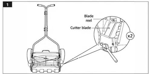
• To loosen the blade reel, loosen rear adjustment bolts on both sides equally by turning them counter-clockwise and tighten front adjustment bolts on both sides equally by turning them clockwise. The cutter blade moves away from the blade reel.
