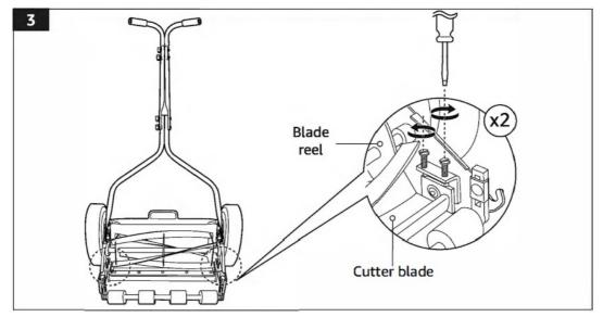
• To check the adjustment, turn the lawn mower upside down. Wearing gloves, take a strip of paper and carefully turn the blade reel so that a blade cuts a small portion of the paper. Repeat for all blades. Each blade should slice the paper evenly across the entire length of the cutter blade while the reel turns smoothly.
