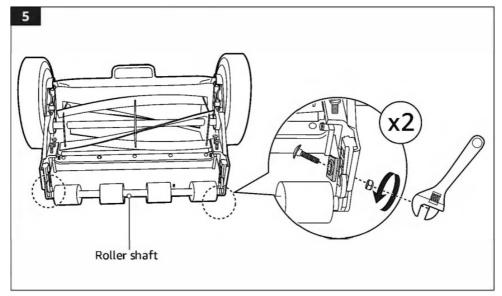
2. Tilt the mower blade forward. Reinsert the roller shaft at an 45° angle .
