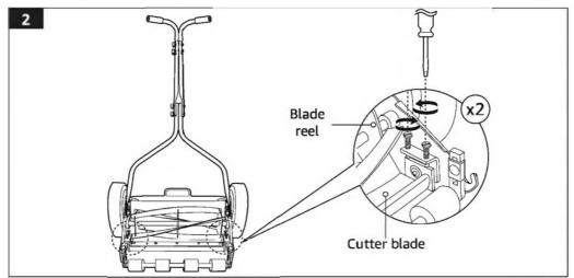
• To tighten the blade reel, loosen front adjustment bolts on both sides equally by turning them counter-clockwise and tighten rear adjustment bolts on both sides equally by turning them clockwise. The cutter blade moves closer to the blade reel.
