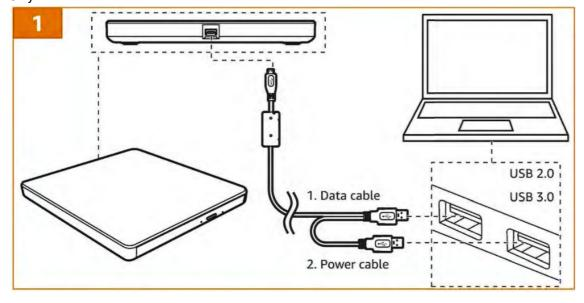
1. Connect a USB-A plug of the USB-A power/data cable (H) to a USB 2.0 or 3.0 port on a compute or laptop (Fig. 1).
