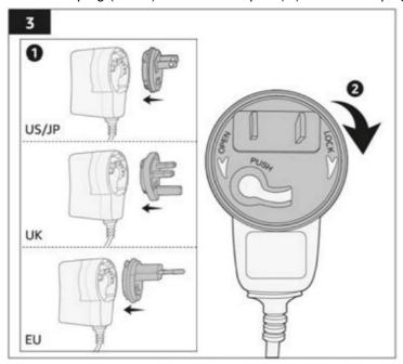
**NOTICE** To detach the plug (R/S/T) from the AC adapter (Q), press the plug release button (U) and rotate the plug (R/S/T) counterclockwise.
