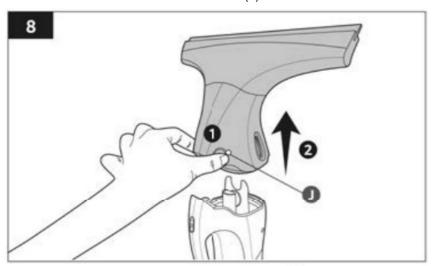
2. Press the suction nozzle release button (B) and remove the suction nozzle (A) from the suction head (C) (Fig. 9).
