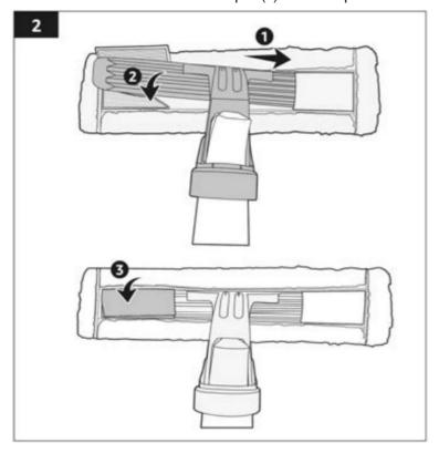
Close the hook and loop closure on the cleaning pad (K).
