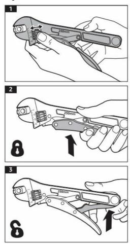
• Press the quick-release lever (3) to unlock the locking handle (2), then turn the worm gear (1) to release the nut (4) from the wrench jaw.
