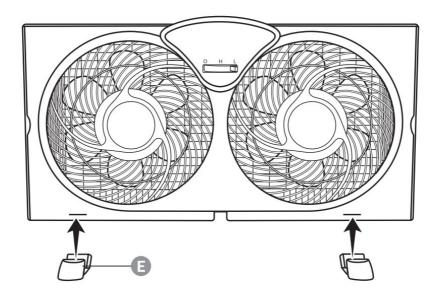
Align the stands (E) with the indents on the main body. Push the stands in until they snap in place.
