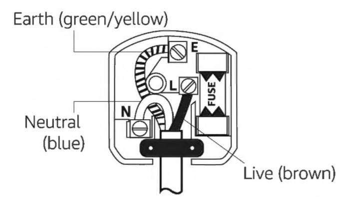
The outer sheath of the cable should be firmly held by the clamp
