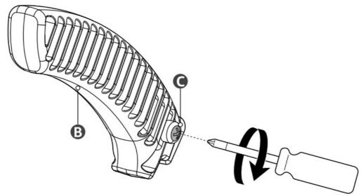
**Step 2:** Fix the handle (B) to the blade latch (D) with a handle screw (C).
