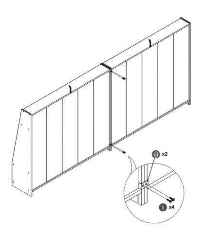
• Use Back Connector to connect if have more than one products (Not necessary).
