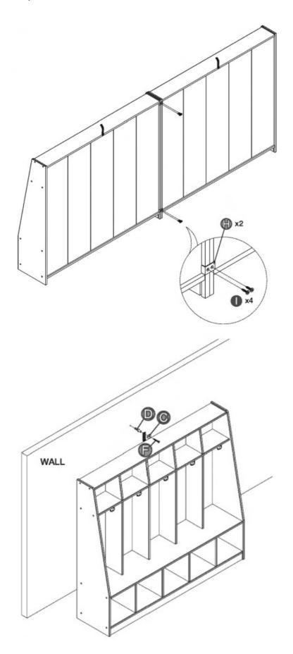
anchor(s) is/are properly installed. Use the appropriate hardware for your wall type.
