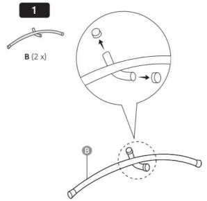
Please remove the 4 protective sleeves before installing the product.
