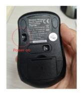
6. Power on switch, Light/ Sensor came on for few seconds Red color and off ,the same time battery power on indicator light on few seconds( power on/off, light
