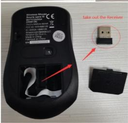
2. Install the battery (take out the battery from the box, check battery + and - and battery size
