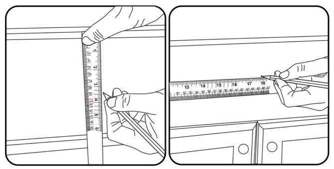
**Step 2:** Measure two opposing marks that extend half the distance of your handle hole centers. For example, if your handle has a 3-inch hole center, mark two points that are 1.5 inches in either direction. Use a level to ensure that your marked locations are straight.
