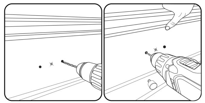
**Step 4:** Align your new handle with the drawer holes. While supporting the handle with one hand, install the handle using the replacement screws included in your pack. Tighten until secured.
