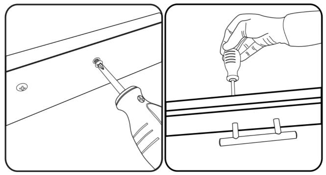
**Step C:** Align your new handle with the drawer holes. While supporting the handle with one hand, install the handle using the replacement screws included in your pack. Tighten until secured.
