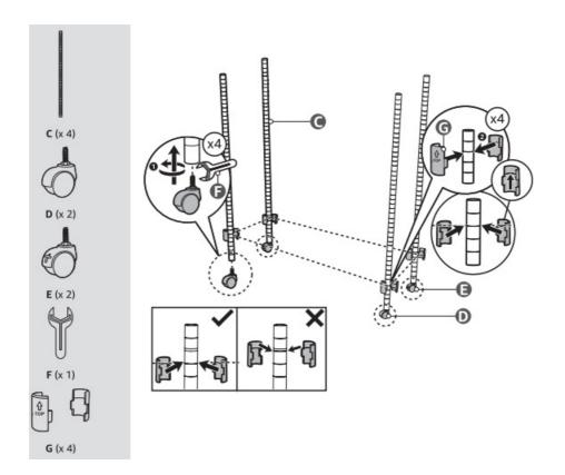
**NOTICE** Make sure lock the sleeves (E) following the TOP side. Match the ridges of the sleeves (E) to the indents on the legs (B/C).
