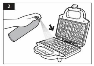
4. Open the appliance and lightly spray or apply cooking oil to the cooking surfaces (F) (Fig. 2).
