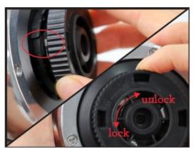
10. If the distributor is installed correctly, a small triangle plate will appear on the top.
