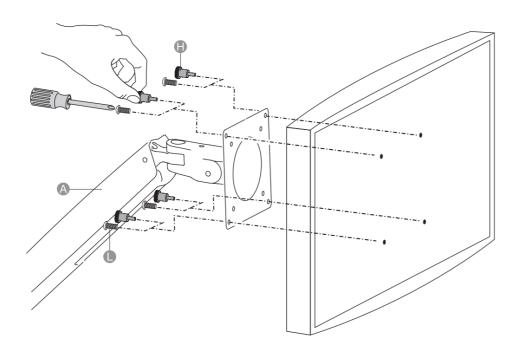
• The arm mechanism is under tension and will move up rapidly, on its own, as soon as attached equipment is removed. For this reason, do not remove equipment unless the arm has been moved to the highest position! Failure to follow this instruction may result in serious personal injury and/or equipment damage.
