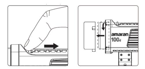
\* **Notice:** Always remove the protection cover prior to turning on the light. Always re-install the cover when packing it away.
