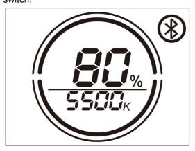
Rotate the CCT adjusting knob to increase or decrease with 100K as the change amount to change the current CCT value (2700K-6500K), and display (2700K 6500K) CCT value in real time on the light body display screen. Click the CCT adjustment knob to quickly switch the color temperature shift: 2700K  $\rightarrow$ 3200K $\rightarrow$ 4300K $\rightarrow$ 5600K $\rightarrow$ 6500K $\rightarrow$ 2700K $\rightarrow$ 3200K $\rightarrow$ 4300  $\rightarrow$ 5600K $\rightarrow$ 6500K cycle switch.
