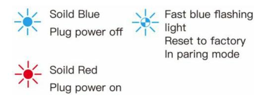
NOTE: Press and hold for 5 seconds to reset the plug to factory setting and put it in paring mode.
