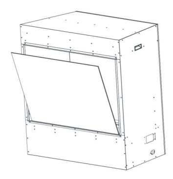
3. Unscrew 6 screws and remove the brackets which are fending the black glass liners.
