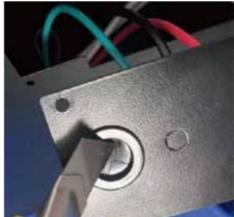
2. Attach the wiring to the junction block. Please make sure the live wire goes into the "L", the neutral wire into "N" and the ground wire into "G".
