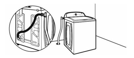
Floor drain system requires a Siphon Break Kit (Part Number 285834), 2 Connector Kits (Part Number 285835), and an Extension Drain Hose (Part Number 285863) that may be purchased separately. To order, please see toll-free phone numbers in your Use and Care Guide. Minimum siphon break: 28" (710 mm) from bottom of washer. (Additional hoses may be needed.)
