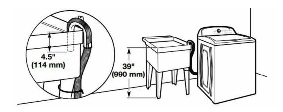
Minimum capacity: 20 gal. (76 L). Top of laundry tub must be at least 39" (990 mm) above floor; install no higher than 96" (2.44 m) from bottom of washer.
