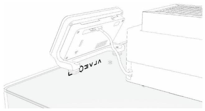
2. Plug the board V2 temperature sensor and put the metal part on the orifice behind the board V2 on the enclosure top surface.
