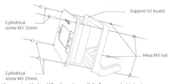
2. Mount the support and the board V2 on the enclosure with the 2 screws and printed pads.
