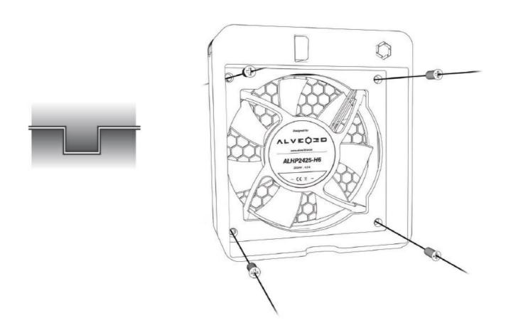
• The head of the self-tapping screws must go a little inside the plastic (to avoid contact with the filter frame), but avoid an excessive tightening.
