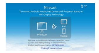
**Step 3**: Activate the Multi-screen/Smart View/Wireless Display function on your Android device and search for the projector.
