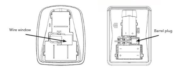
• Insert the Keypad into the table stand. Push any extra wire into the stand before inserting it into stand. Slide the Keypad on stand until it "clicks" into place.
