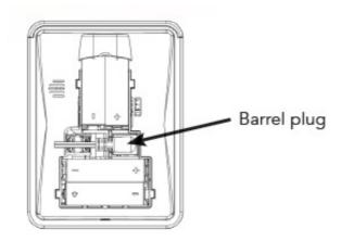
• Insert the Keypad into the mounting plate. Push any extra wire behind wall plate before inserting into mounting plate. Slide the Keypad on plate until it "clicks" into place.
