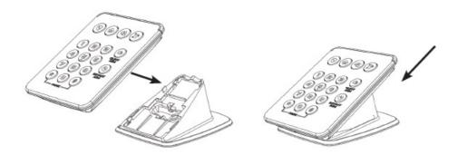
• Coil up the excess power wire into the stand. Insert wire into wire holder and close stand cover to contain excess wires.
