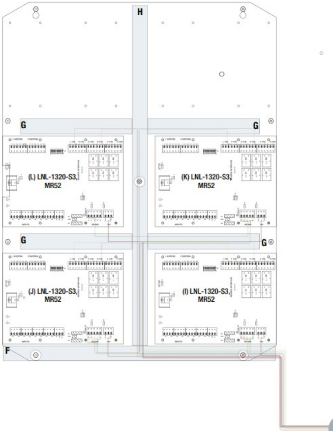
TMV2 – Door Backplane accommodates four Mercury boards
