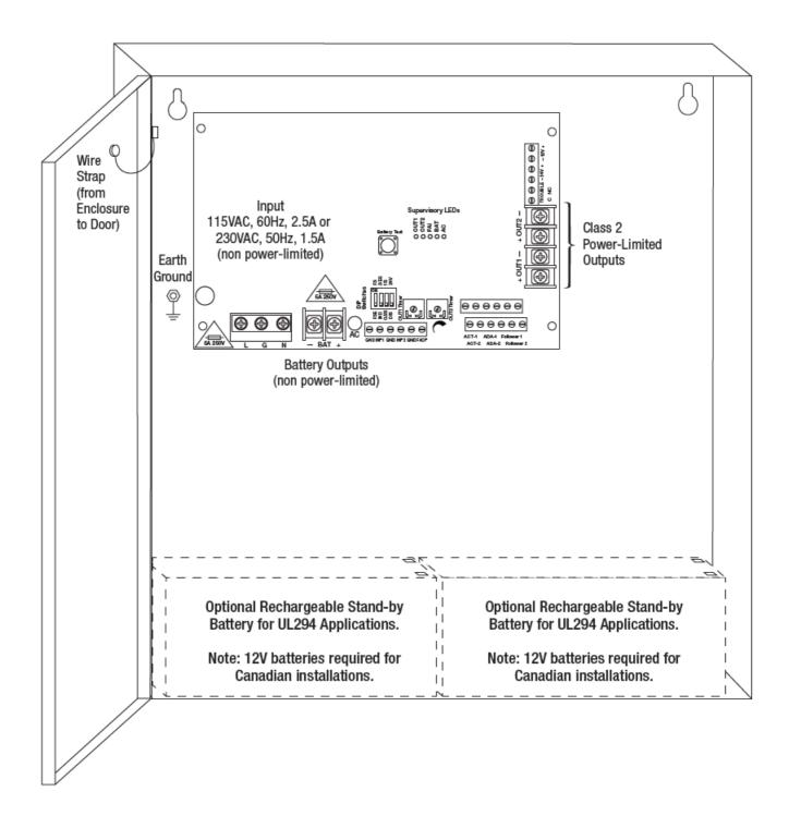
Keep power-limited wiring separate from non-power-limited. Use minimum 0.25" spacing. 7AH Rechargeable batteries are the largest batteries that can fit in this enclosure (UL/ULC – Stand-by power only evaluated with 7AH batteries). A UL-Listed external battery enclosure must be used if using 12AH, 40AH or 65AH batteries.
