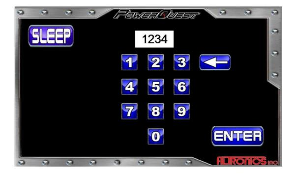
Master Code: On the back of Module (not the touch screen) there is a tag with the systems Master 4 digit program code and a Temporary User Code. You can use the Master code to program your User code. The Master code can always be used to reset User code.
