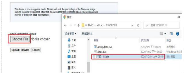
• Press "Choose File" to select the BMC firmware, xxxxx.bin. Then press Open to upload the BMC firmware.
