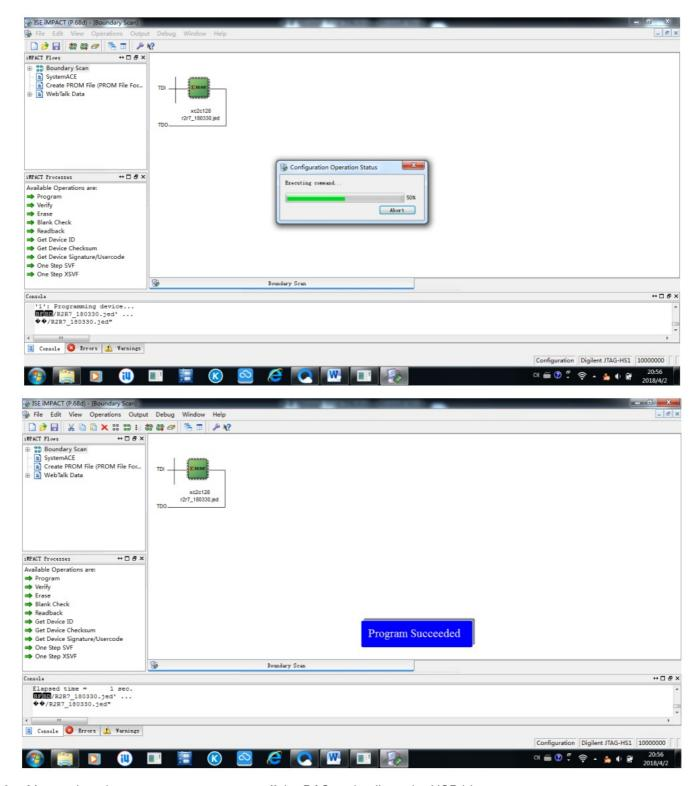
8. After update the program, you can turn off the DAC and pull out the USB blaster.
