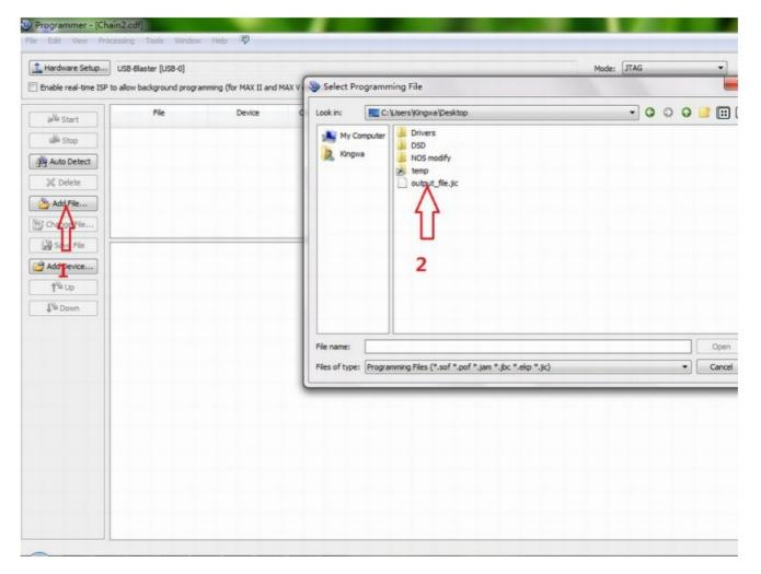
8. Follow the steps select as below, you can see the two chip diagrams in the bottom window, the chips should show their model name, like "EPCS4 and EP2C8 or EP4C10". (If the chips' name unshow, it most like the blaster output wires has bad connect, you had to power off the DAC, pull and push the blaster output wires, then power on the DAC).
