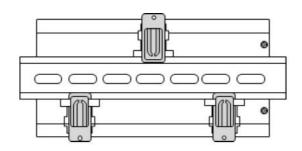
To install the controller onto a DIN mounting rail, from the fully pushed in position slide the top mounting foot out by 2 clicks so that the foot is clear of the DIN rail channel. Slide the bottom two feet out by one click so that they are protruding slightly into the DIN rail channel. The controller can now be inserted onto the DIN rail by inserting the bottom lip of the DIN rail behind the two bottom mounting feet.
