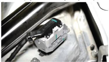
2. Access the Frunk and re-connect the low-voltage battery connector.
