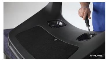
4. Re-use the factory screws to install the new speakers EV-40M-T. Re-attach the grilles to the panel by bending the tabs into place. Install the 2 factory plugs to each speaker.
