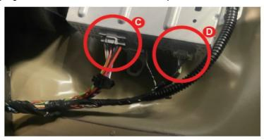
• Route the Alpine harness cable along the factory wire channel, toward the B-Pillar. Make sure the wire is properly tucked
