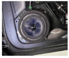
5. Plug in all remaining factory door connectors. Mount and re-install each factory door panel using (3) T30 Torx.
