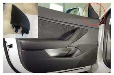
2. With the Tweeter Housing un-clipped from the door unplug the factory speaker connector. If the plug is difficult use a small precision flat tool to release the plug connection.
