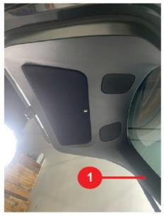
2. Using a panel tool release the panel from the body of the vehicle. Pull out and unplug the single connector from the panel. The hatch panel should now be able to be removed outside the vehicle
