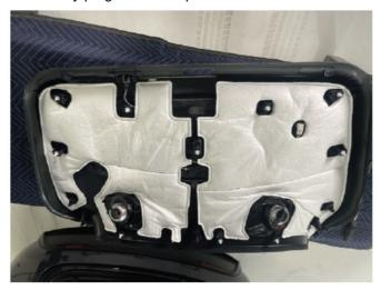
5. Reconnect the factory plug and Install the panel with new speakers into the hatch by aligning and applying pressure to push clips. Lastly, install the 2 pillar push pins and upper pillar shrouds.
