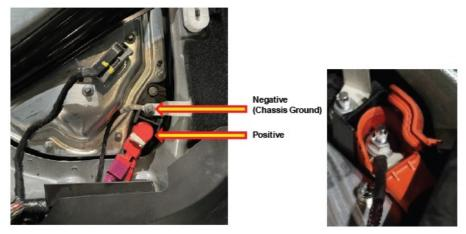
4. Route 12V Power Harness (Plug J) from the rear bench seat to the trunk to the amp mounting location.
