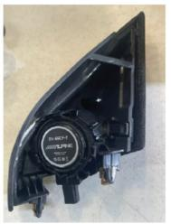
5. Plug in the original factory connector to the new Alpine tweeter and pop the housing into place using downward pressure along the factory clips. Make sure it securely latches into place.
