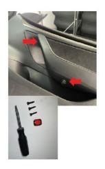
2. Use a Panel Removal Tool around the edge of the panel to release the factory clips. Release the panel and pull upwards to detatch, unplug the factory panel connec-tions including the green speaker plug.
