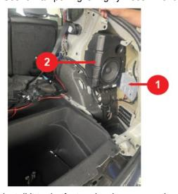
3. Mount the new subwoofer box and install it to the factory hardware mounting positions. Next re-fasten the factory amplifier using original hardware.
