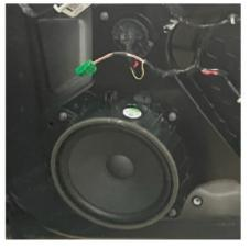
4. Install the new Alpine Speaker & Adapter to the door panel using the factory screws. Plug in the green factory speaker adapter plug.
