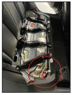
3. Connect the Alpine harness Positive and Negative lug to the low-voltage battery posts under the rear seat & retighten the hardware.
