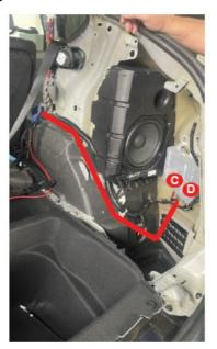
• Disconnect two factory plugs from the rear amplifier and replace them with the alpine harness plugs (C+D). transfer the original car plugs back into the female end of the Alpine Harness
