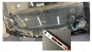
4. If your vehicle is equipped with a center speaker connect the Y-Harness between the center mid and tweeter & Plug all speakers into the factory connectors
