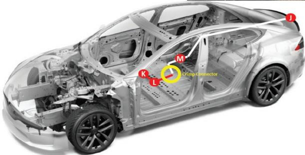
5. When finished tuck all excess wiring and CANPRO module into the rear center console compartment and reinstall the lower cover using factory clips.
