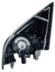
4. Install the new Alpine Tweeter to the housing by positioning the lock tabs and clipping them into place.
