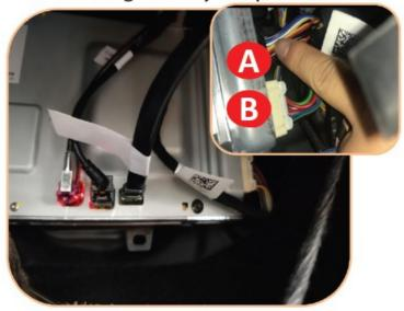
• Route the Alpine harness cable along the factory wire channel, toward the B-Pillar. Make sure the wire is properly tucked
