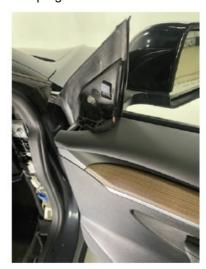
3. Unclip the Factory Tweeter from the Housing by gently twisting and pulling.
