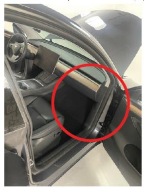
• First, remove the under-dashboard trim panel (#1) by releasing all retaining clips and pulling.
