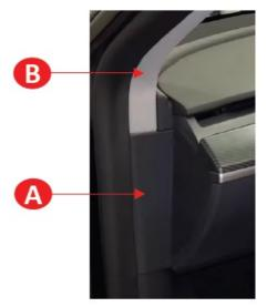
2. Use a Panel Removal Tool around the edge of the dashboard speaker cover panel to release the factory clips. Release the panel and pull upwards to detach and expose the center stage speakers.
