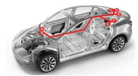
• Loosen the base of the B-Pillar Panel and route the harness from the front half of the vehicle towards the rear
