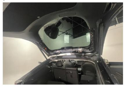
3. Disconnect the speaker plugs from each factory speaker. Un-bend (9) tabs in each grille to expose both speaker mounting flanges. Using a T25 Torx bit undo 3 screws from each driver and remove the factory speaker.
