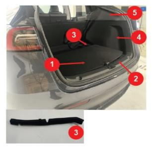
2. To make room for the new subwoofer #1 Dismount the factory amplifier (2 Nuts 1 Bolt) 10mm #2 Remove the factory subwoofer (3 Bolts) 10mm \*Sound Dampening is Highly Recommended at this stage.
