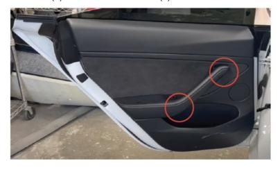
2. Use a Panel Removal Tool around the edge of the panel to release the factory clips. Release the panel and pull upwards to detatch, and unplug the factory panel connections.
