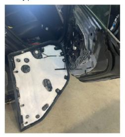
3. Using a Drill Bit, Drill out 3 Plastic Rivets on each Factory Door Speaker. Use Care to not over-drill the screw boss.
