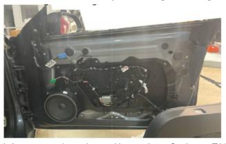
3. Remove 4 bolts securing each factory speaker adapter. Use an 8mm Socket or T25 Torx (Varies depending on the year) The factory Adapter should then unclip easily.
