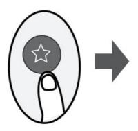
Push this button when remote controller is on, the system will automatically revert back to the previous settings including operating mode, setting temperature, fan speed level and sleep feature (if activated). If pushing more than 2 seconds, the system will automatically restore the current operation settings including operating mode, setting temperature, fan speed level and sleep feature (if activated).
