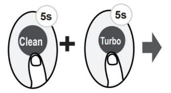
Press together Clean button and Turbo button at the same time more than 5 seconds to activate Lock function. All buttons will not response except pressing these two buttons for two seconds again to disable locking.
