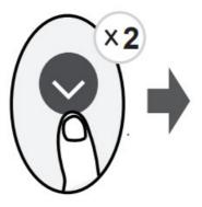
Keep pressing Fan button for more than 2 seconds to activate/disable Silence function(some units). Due to low frequency operation of compressor, it may result in insufficient cooling and heating capacity. Press ON/OFF, Mode, Sleep, Turbo or Clean button while operating will cancel silence function.
