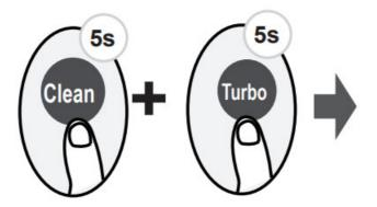
The unit will operate at high fan speed (while compressor on) with temperature automatically set to 8 C/46 F.
