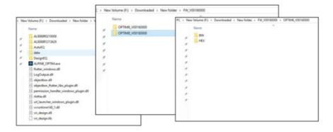
1-5 Inside the BIN folder for the PXE-C60-60 is a file that is called AutoEQ2.0\_CSP6\_Ver1.600000\_0822.bin. The PXE-C80-88 has a file called AutoEQ2.0\_CSP8\_Ver1.600000\_0823.bin inside of it. Those are the firmware files that will need to be selected in the later steps. The first picture shows an example of this.
