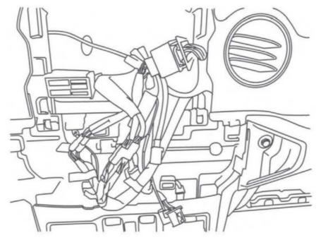
10. Connect the replacement dash speakers and mount them using the factory screws.
