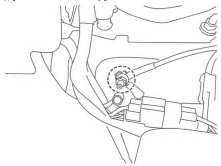
7. Connect the main harness to the amplifier assembly and align it to the seat mounting holes.
