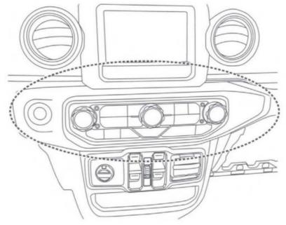
3. Extract (2) 7mm/Phillips screws on the bottom of the radio bezel.
