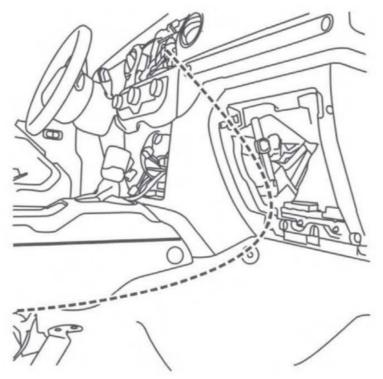
9. Connect the T-harness and main harness to the radio. Refer to page 8, 9 or 10 for the corresponding system wiring diagram.
