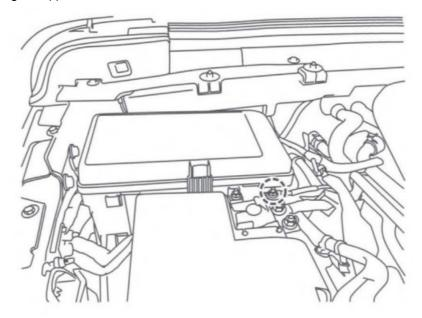
2. Route the power cable following the factory harness along the vehicle's frame.
