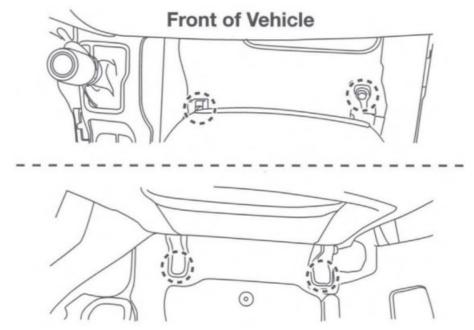
8. Tilt the passenger seat towards the back to reveal (2) connectors, disconnect and remove the seat.
