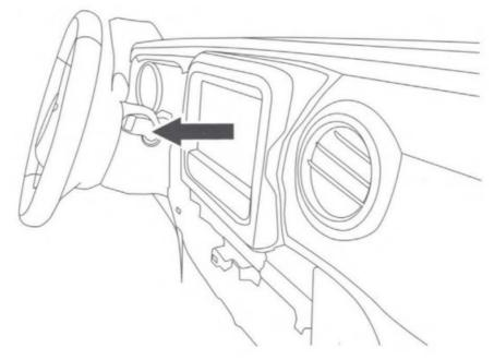
5. Extract (4) 7mm/Phillips screws from the factory radio, disconnect and remove it.
