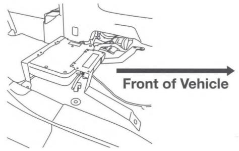
8. Route the main harness along the side of the center console to the radio location.
