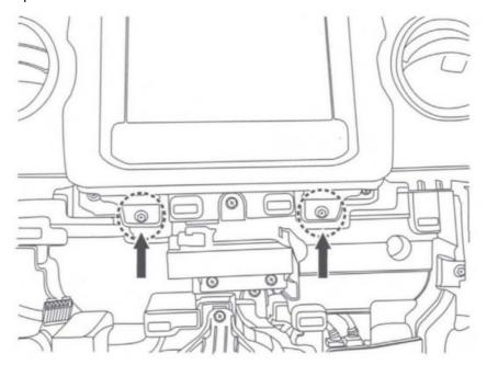
4. Use a panel removal tool to release (6) clips on the radio bezel and remove it.
