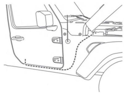
3. Route the Positive(+) power cable through the grommet under the carpet and pull the power cable from under the vehicle. **Note:** seal the grommet with silicone (not included) to prevent water from entering the cabin.
