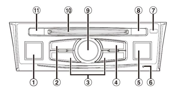
(AUDIO)/(Favorite) button: Displays the Audio/Visual screen. If the Audio/Visual screen is already displayed, changes the source. Press and hold for at least 2 seconds to recall the Favourite screen.
