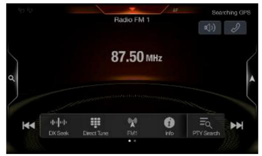
6. Then the second phase of the software update takes place. Press the "OK" button when an update message appears on the screen. The process will now install the new map data and navigation application data to your Alpine Head Unit.
