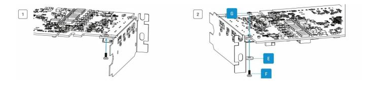
• Use the original screws of the graphics card (1) and use the screws supplied in the accessories (2).
